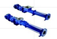
Max. Capacity: 140 m3/hr Max. Pressure: 24 bar Max. Viscosity: 1,00,000 cSt Material of Construction Body: Cast Iron / Carbon Steel / SS Rotor: Tool Steel / Stainless Steel Stator: Natural Rubber, Nitrile, Neoprene, Hyplaon, EPDM, Viton
